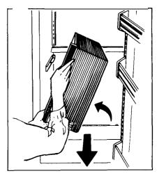
8. Tilt and remove the drawer. After cleaning, replace in reverse order.
